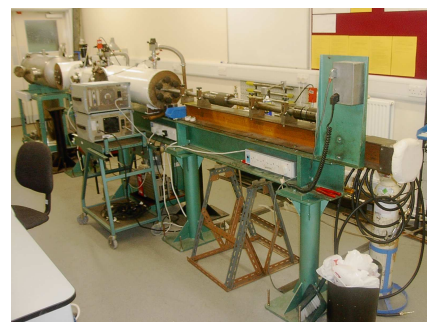
The two stage light gas gun on which Professor Burchell conducted his experiments, in the School of Physical Sciences.
