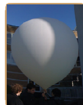
Sounding balloon that was filled with helium
