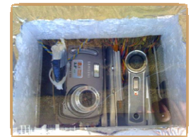
Payload—2 digital HD cameras
