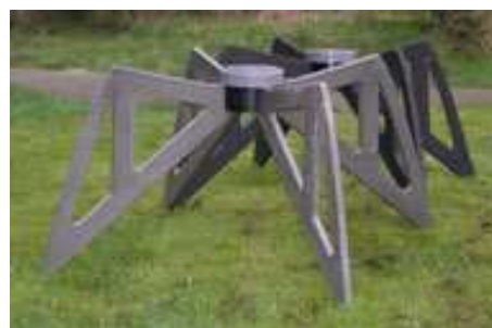
The High Band Antenna can be used between 120-240 MHz. The FM band is suppressed in the antenna amplifier for both antennas to minimize intermodulation products from FM transmitters. This antenna is a composite system consisting of 4x4 dual-polarization dipoles and a dual-polarization RF beamformer
